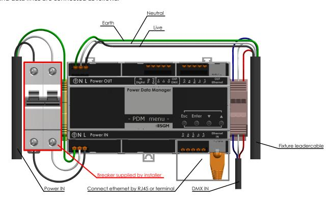
Ensure High Voltage and Low Voltage cables are kept separate where possible. Connect earth/ground wire first.
